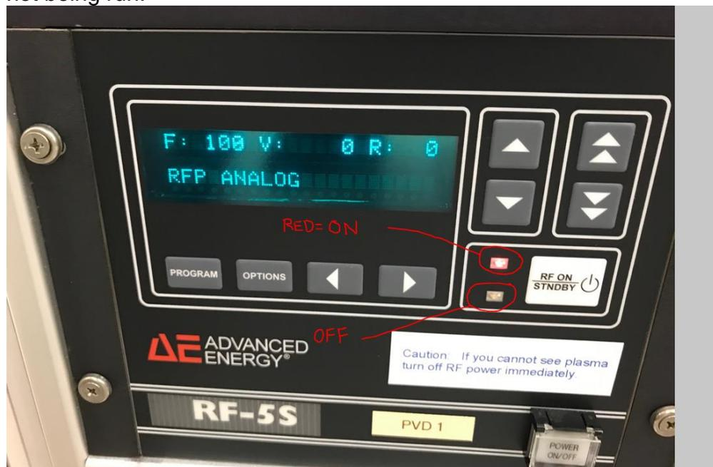
Open the front door to the tool and check if the RED light on the RF-S5 power supply is ON. If on, wait until the clean process is complete before logging on to the tool. Cleans usually last no more than 30 minutes.
