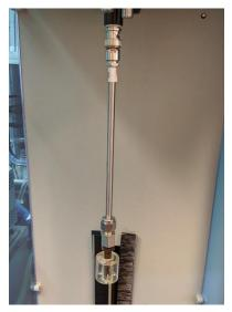
With this configuration we will not use the thermometer, but will instead use the float sensor, the float sensor should be place on the same connection that you would typically place the thermometer. This will ensure the cells are submerged in the cooled water during the experiment and should keep the dewar from lifting far enough to contact and damage the cells.
