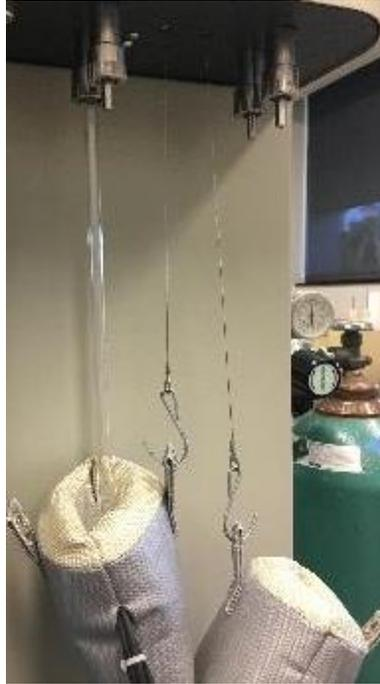
9. Remove empty cold trap Dewar from the outgassing station and fill cold trap Dewar with liquid nitrogen (use cryogenic gloves and face shield for safety precautions).
