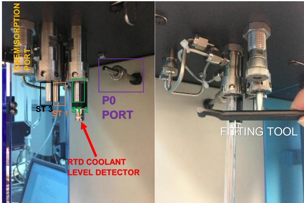
8. Engage the coolant level sensor (RTD) in the analysis station.
