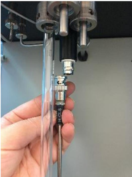
9. Remove metal pin from the P0 port, then attach Po in the analysis station. P0 cell is used to measure the saturated vapor pressure of adsorbate, or substance adsorbed, during an analysis (e.g. Nitrogen).
