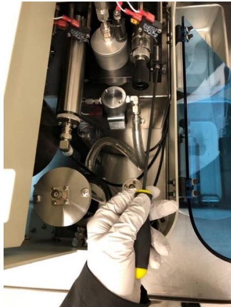
Figure 10. Overhead view of changing angle adjustment screw for macro cell
