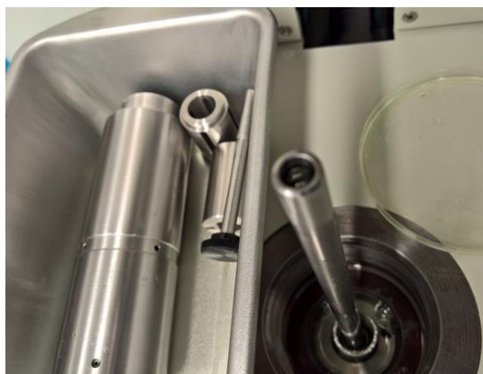
Figure 26. Macro cell in high pressure chamber
