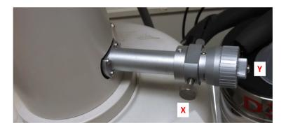
Move knobs until image no longer moves Up/Down and Left/Right. When the aperture alignment is complete, close the alignment menu and the image wobble will stop.
