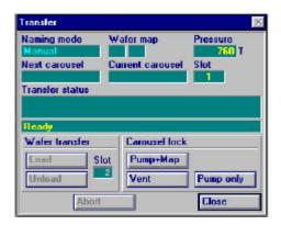
The carousel loadlock will vent to atmospheric pressure. When the carousel loadlock is at atmospheric pressure, the operator will be prompted to open the carousel loadlock lid and load the carousel
