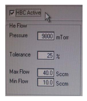
The helium leak up rate test parameters are set in the HeLUR tab; max should be 20 to 25 mTorr/min. LURs over 10 will however will cause process variation, a clean fresh wafer should be in the 5 to 6 range.
