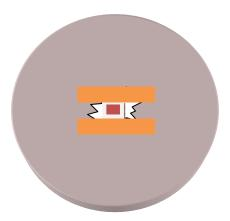
Example of a carrier wafer with the small piece is adhered with heat sink compound and two of the four needed pieces of polyimide tape are in place.
