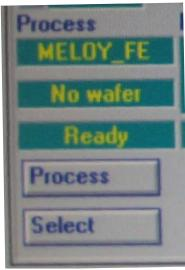
**NOTE:** Never command the machine to do anything unless the word "READY" appears in the lower left part of the Operators Station window. Failure to do so will cause the software to lock up.
