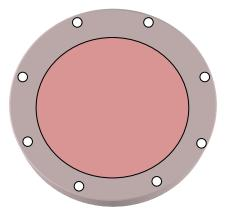
This has the effect of creating a flower petal pattern outside the uniform zone. The center area is the most uniform. The white dots are where the wafer clamp contacts and are slightly cooler than the outside edge. The hottest portion of the wafer is the outside edge at the midpoint between the wafers clamps.
