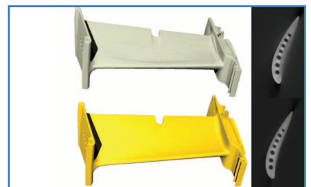
Up to 300 kV high power scans (below) ensure reduced artifacts e.g. for turbine blade inspection tasks
