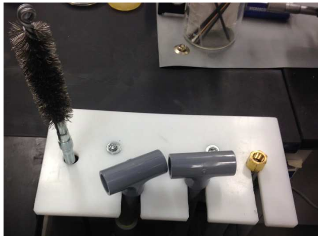
Figure 17 Flue Brush Storage Behind System
