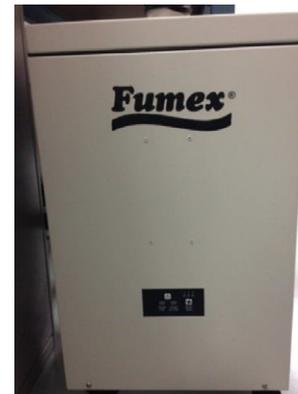
4. Using air velocity meter provided, verify the velocity in the center of the closed lid is  $> 3$  m/s [600 ft./min]. If air flow does not meet specification **do not** continue with this work instruction.
