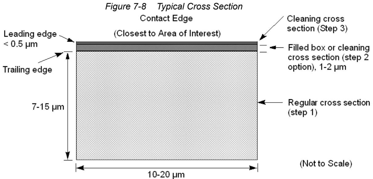
Be attentive to boxes positioning if you are sectioning a specific point. Use fine milling to expose the exact area of interest. For example, a 2  $\mu\text{m}$  offset should be more than enough at 3 nA of current. Calculate the outline as the height of the box relative to the depth to be milled. If you intend to view at 52° and see details 3  $\mu\text{m}$  from the surface, then the original box should be at least 3  $\mu\text{m}$  tall.
