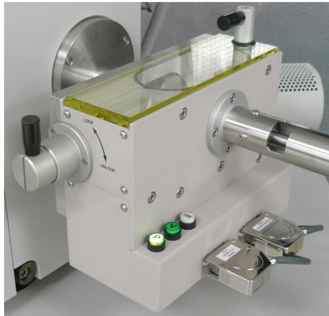
The loader consists of a loading rod with set slide and parking position, a vacuum chamber for loading and unloading the sample carrier (with sample) onto a bayonet fitting located at the end of the rod. A gate valve seals the vacuum of the SDB / SEM specimen
