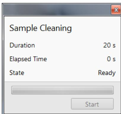
For avoiding typical “weak” contamination artefacts during high resolution imaging (image darkening), 1-2 minutes plasma cleaning duration in combination with cryo cleaning (see “CryoCleanerEC” on page 380) should be sufficient. When bulky deposition is visible (mostly on image corners), 5 minutes duration is recommended.
