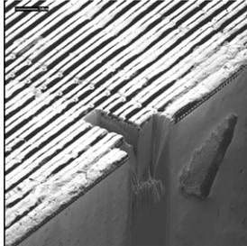
Perspective view of the cross section milled on the edge of a sample
