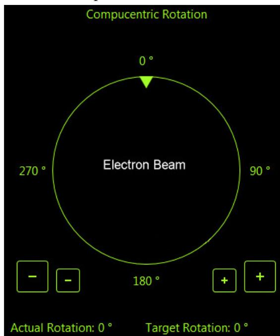
By clicking and holding the mouse button down on the green triangle, it can be moved around the circle to choose a new orientation of the sample relative to the detection position. On release of the left mouse button, the computer software updates the position orientation and offset from the mechanical stage center to deliver the same object center, but rotated to the angle selected.
