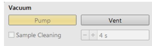
When in operation, the electron source and column section are always under high vacuum. The specimen chamber is at the pressure required for the given state (Pump / Vent) or mode (HiVac / LoVac / ESEM).
