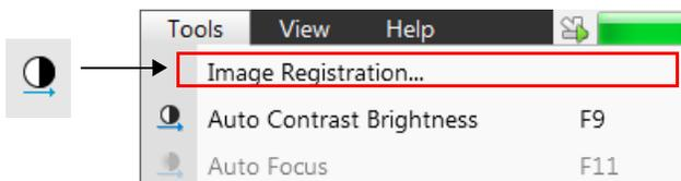
The system will attempt a correction of the contrast and brightness levels to suit the sample so that the majority of graylevels are shown. When activated, a dialog box appears to show the progress of the function.
