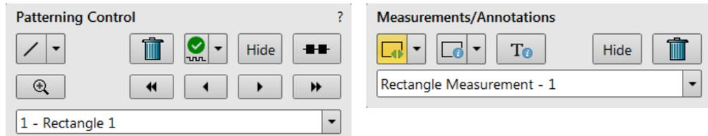
A Pattern, Measurement or Annotation can be drawn and modified (focusing, moving, or resizing) by the toolbar functions in the same way. This gives a user many capabilities to draw pattern shapes, to measure distances, angles, diameters and areas as well as locating and labelling items that are of significant interest on the sample area.
