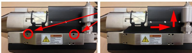
18. Release the Viton band from the chamber door and remove the MultiChem chamber cover.
