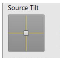
Click on the 2D box and hold down the left mouse button; a cross-hair shows onscreen with a small 4-ended arrow cursor located in the center. By moving the mouse, the cross-hairs move and affect the image as required. Due to the fact that the probe rotation correction is switched off automatically in some alignment procedures, the X and Y movements may not always appear to be in the same directions.
