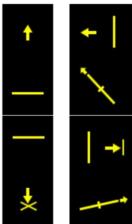
When a yellow line perpendicular to the moving direction appears, the stage approaches the movement limit in that direction; when a yellow cross appears, the limit was reached.
