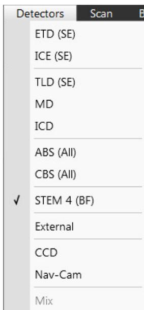
When a detector mode is selected, its acronym shows to the right of the detector name in the menu. In addition to the standard detectors available, there may be optional ones available for your system type.
