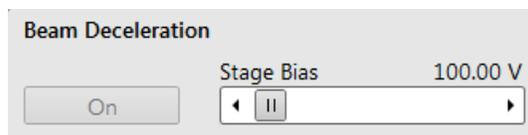
At low magnifications, an ETD image should become dark symmetrically around the window center; in other cases, the sample could be tilted. When a dark area is shifted with a stage bias change, the sample is possibly not parallel with the detector. Use compucentric stage rotation/stage tilt to keep the dark are in the center of the screen.
