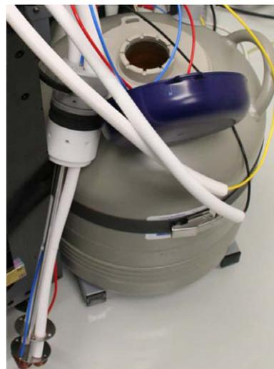
The insulated pipes coming out of the central core then proceed to the gas flow and electrical interface flange situated on a chamber port.
