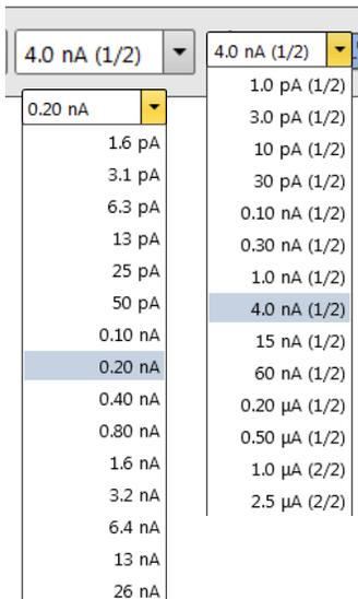
The maximum E-beam current for the UC mode is 100 pA. The aperture holes for the FIB wear out with regular use so multiple apertures are available for commonly used beam currents, which is noticeable by doubling the beam current value. Thermo Fisher Scientific service engineers can mark certain apertures unavailable for use. Unavailable apertures are marked in the beam current list with -...- so they cannot be selected.
