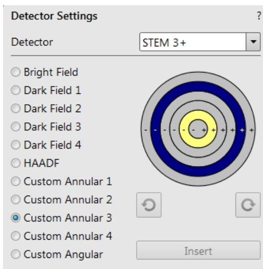
Some combinations of pre-defined (BF, DF1..DF4, HAADF) and Custom modes does not allow simultaneous imaging in all four displays.
