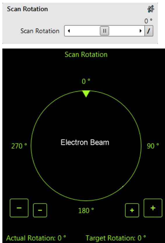
When patterning is in progress, the scan rotation overlay control is restricted only to the - / + buttons.
