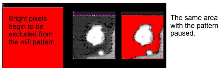
4. Monitor the bright and dark areas while the pattern is milling by adjusting the selected mill pixel range (red bar) either while it is milling or when it is paused.
