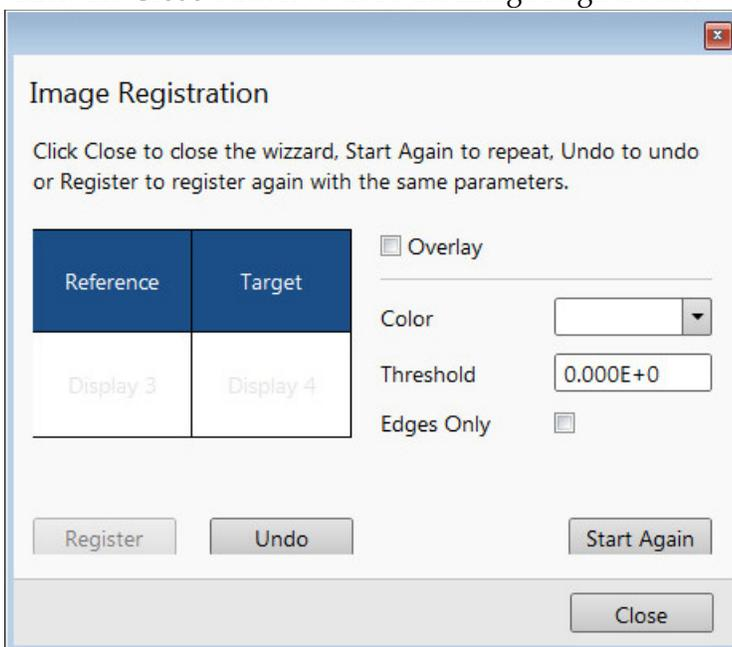
Click the **Start Again** button to repeat the procedure in the same way with the changed (or another) target and reference images placed in the same or different displays. Clicking the **Undo** button restores the image to the situation before the last transformation.
