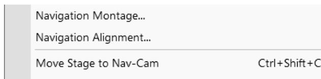
At this moment the beam and the detector changes to Nav-Cam and a live image of the navigation camera is obtained in the last used active display (with the resolution of 768 × 512 pixels only).
