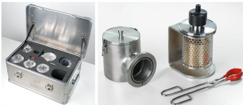
When the specimen chamber (together with the CryoCleaner) is pumped, liquid nitrogen is introduced to the nitrogen vessel. Its outside cold surface absorbs contaminating products from the
