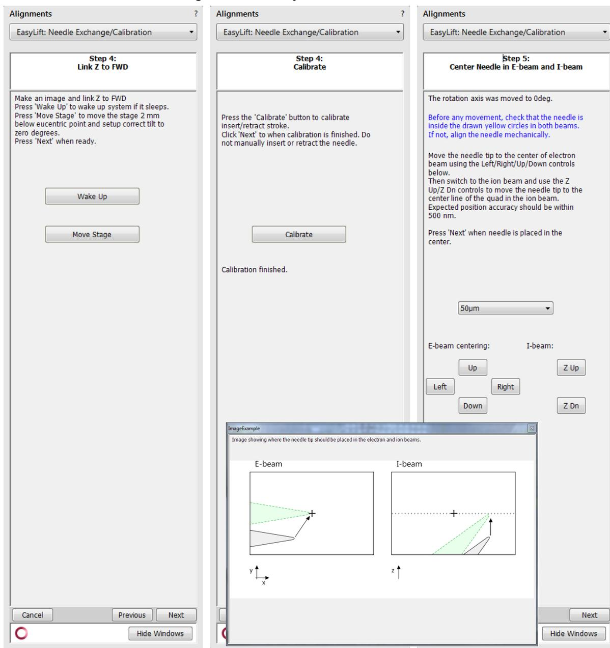
Figure 6-5 EasyLift: Needle Calibration (continuing)
