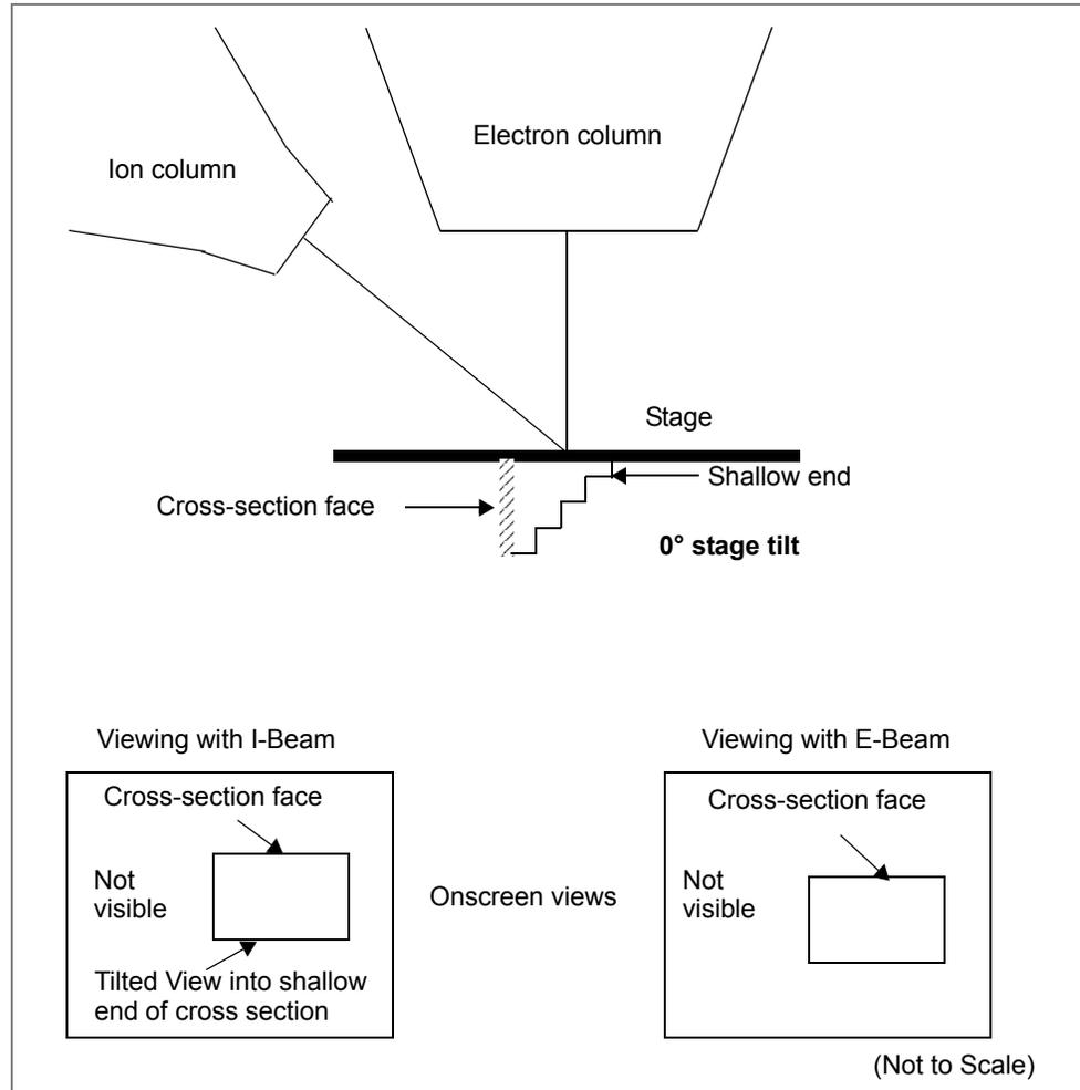
The following image shows the onscreen views with the stage still at 0° tilt, but with both stage and scan rotation at 180°.
