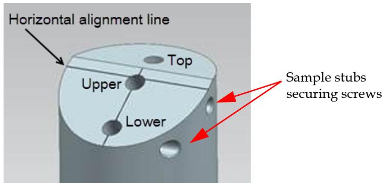
5. Rotate the stub, so that the top of the sample is on the lower side of the slope. Try to rotate it to the desired angle of the sample.
