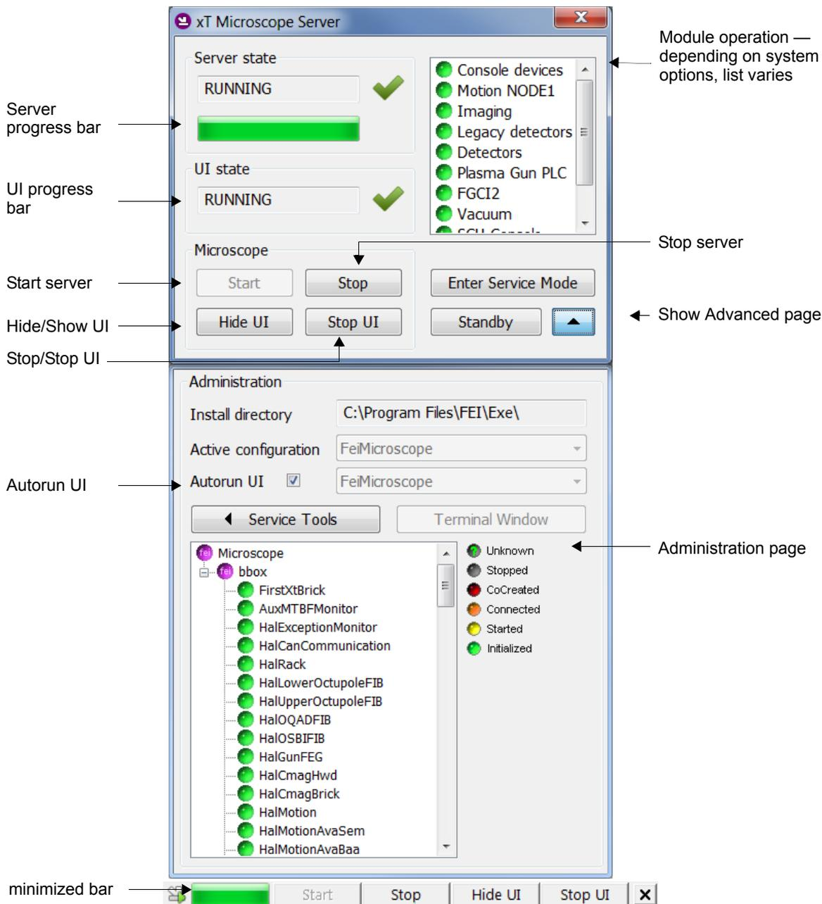
The Startup dialog can be minimized once the UI is established by right-clicking in the top bar of the dialog. This opens another dialog box that offers the chance to minimize the Server to the top bar of the UI. Double-clicking the xT Microscope Server header has the same functionality.
