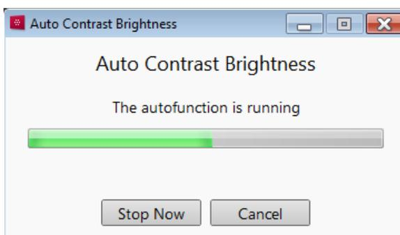
The function can be interrupted by clicking on the **Stop Now** button. This will leave the image at the stage of progress at stopping. Clicking **Cancel** before the function ends will return the image back to its original status.
