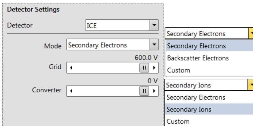
The Electron beam and Ion beam imaging (distinguished by the beam icon in the module header) have different Modes.
