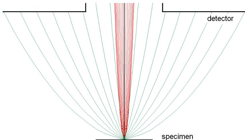
Detectors most convenient for beam deceleration are BSE types placed closely under or directly inside the column. Their efficiency depends on their active area: the smaller the active area's inner diameter the better. The standard ETD could also be used, but its efficiency is low.
