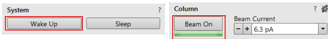
The high voltages are also switched on, the CIVs are opened, and the GIS heaters are turned on.
