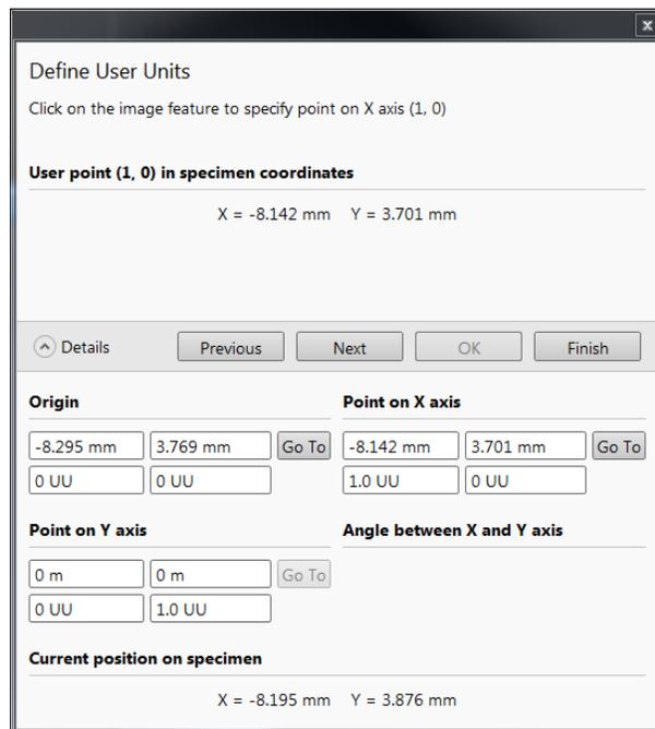
Follow the instructions in the dialog to move to a point and click on it. The coordinates of that point (0,0) appear next to the User X and User Y readout positions in the Details section of the dialog.
