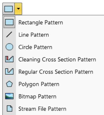
1. On the Patterning module or on the toolbar, select a pattern from the Pattern Selector and draw a pattern in the active display. When the selection is made, the blank area shows the relative icon, as shown.
