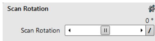
This preset/continuous control adjuster gives access to set rotation angles as well as a variable angle values.
