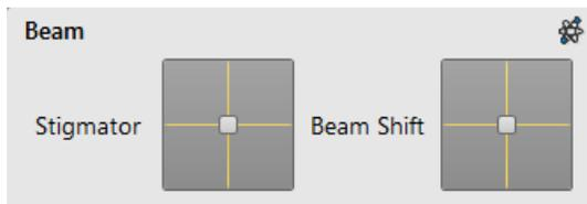
Clicking and dragging anywhere inside the box changes the active display cursor to the 4-ended arrow and positions it to the screen point corresponding to the actual control value (minimum in the middle of the screen and maximum at the edges). It can be dragged in four directions. To fix the values, release the mouse button.
