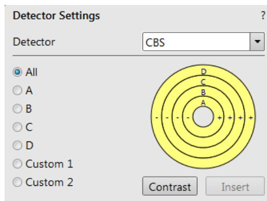
Custom mode is used to define the segments to be used for detecting.
