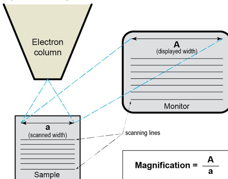
If the size of the raster on the sample is made smaller while the raster on the monitor remains constant in size, the magnification of the image increases.
