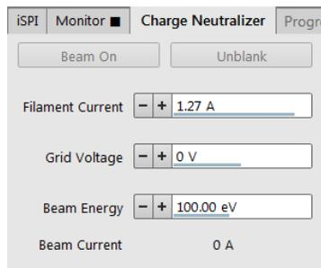
The I-Beam Charge Neutralizer uses a low energy electron beam to control charging induced by the ion beam. This allows imaging and patterning of nonconductive materials and reduces electrostatic discharge-related sample damage (by spreading electrons on the sample).
