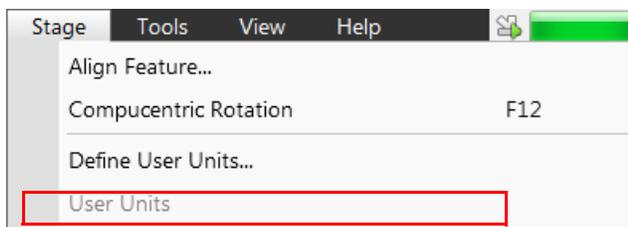
A tick mark appears next to the label. The stage coordinate system reverts to the last defined user unit configuration for 1-, 2-, or 3-point alignment. From this point on, the stage can operate in Absolute or Relative mode with User Units to perform specific movements.
