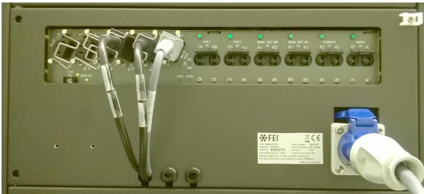
Output power sockets are used for other microscope optional equipment.
