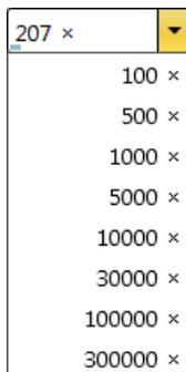
2. Click on the required magnification and it appears in the text box, and the dropdown list automatically closes. This can be done while the beam for the column is on, in which case the change is immediate.
