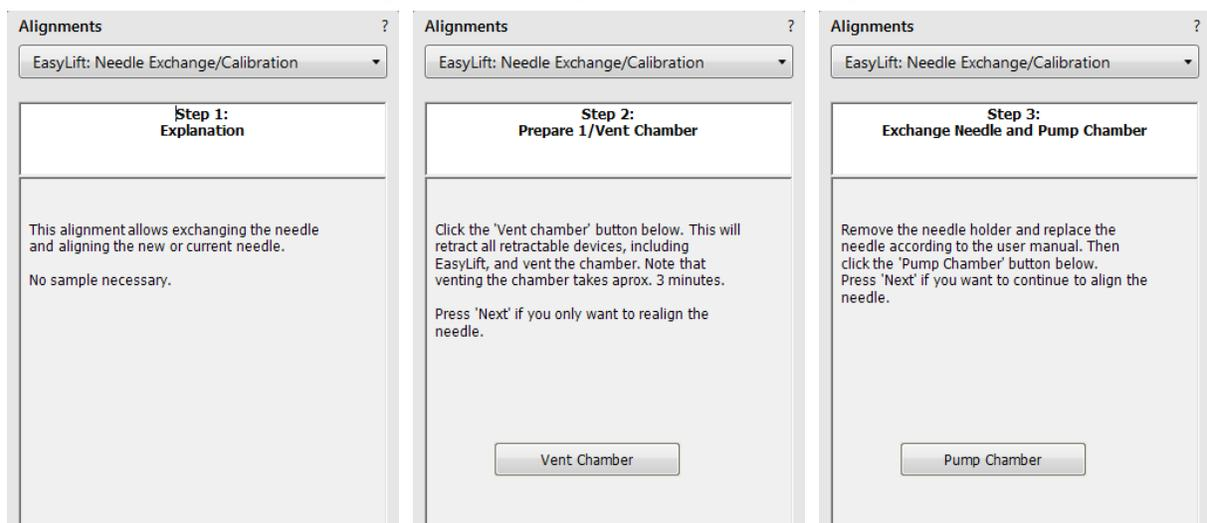
1. **Step 2:** Click the **Vent Chamber** button and wait for the chamber to be vented.
