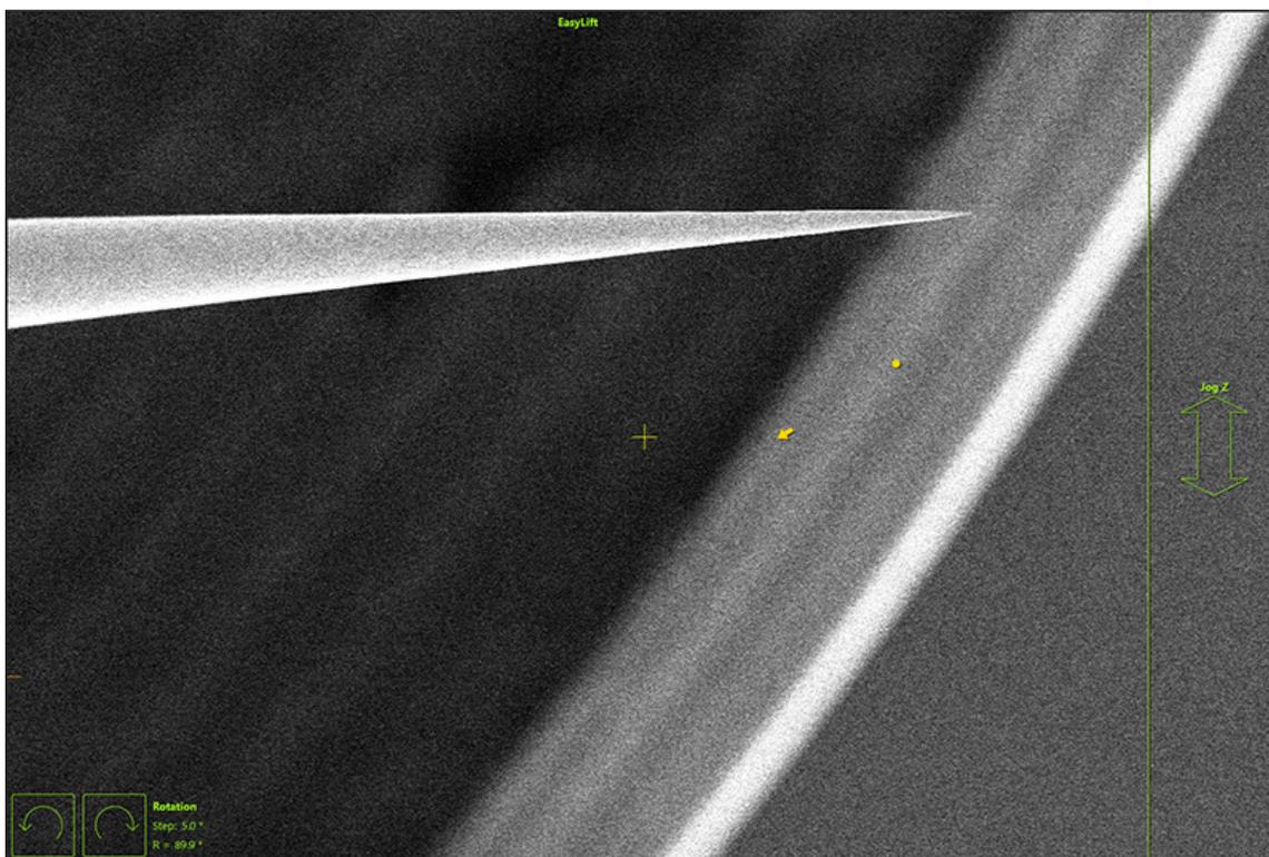
3. Click and drag inside of the arrow area on the right side of the display to move the manipulator in z. Look for Z motion in the ion beam.
