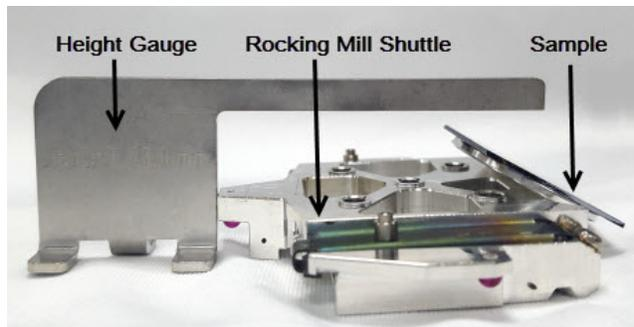
3. Rotate the stub so that the top of the sample is on the lower side of the slope. Try to rotate it to the desired angle of the sample.
