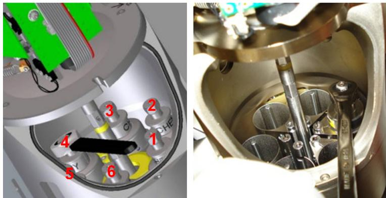
When using the crucible ratchet to install / remove crucibles, place the ratchet end over the hex portion of the crucible and tilt the ratchet up. This will wedge the ratchet to the crucible and keep the wrench from sliding off.
