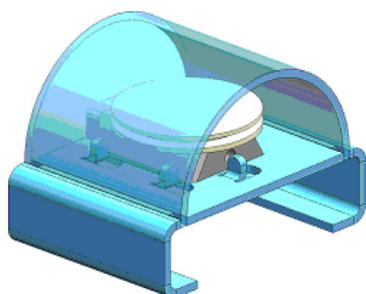
The shuttle clamps with a spring in the dovetail shaped slot of the adapter. It is fixed to the loader arm via a bayonet coupling. The maximum pin length of the stubs that can be used is 11 mm (most
