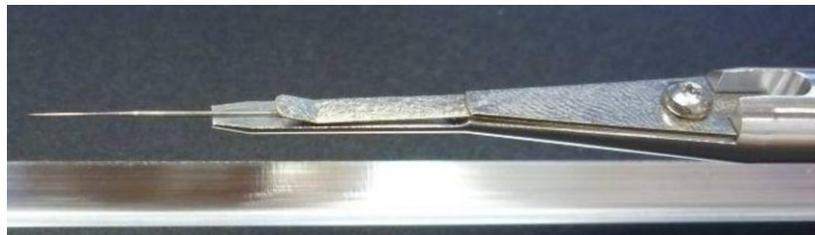
8. Check by rotating the Probe shaft using the knob at the end if the needle is positioned straight. Reduce the needle tip wobbling (should be within 500  $\mu\text{m}$ ).
