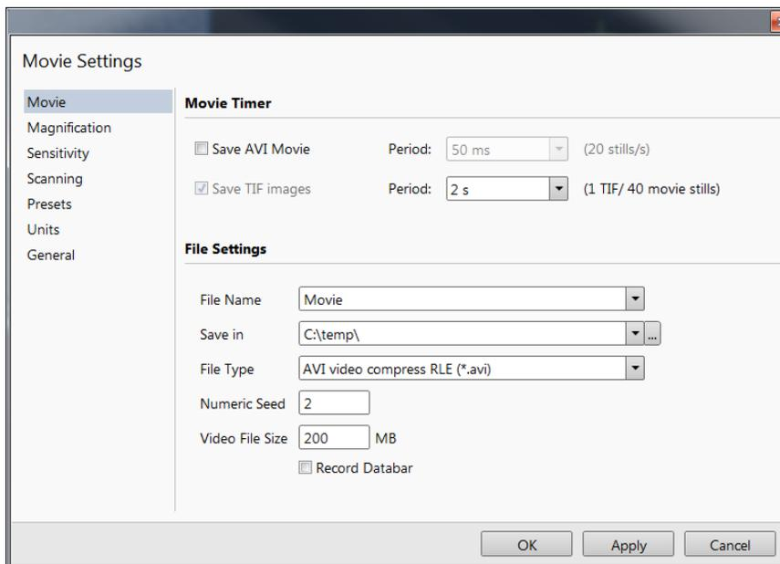
2. In the **Movie Timer** section, tick the **Save AVI Movie** check box and select the desired time from the **Period** dropdown menu. Tick the **Save TIF images** check box, if required, and then a desired **Period**.
