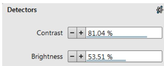
Regardless of the detector actual gain range, the contrast and brightness range is always 0 - 100 (%) and the small/large step size is 0.1/1 (the brightness step size may differ for some detectors in order to achieve a sufficient sensitivity).
