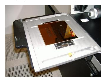
4.4 Flip the mask holder over and slide it into the machine. Lock the mask holder slide by pressing CHANGE MASK key again.
