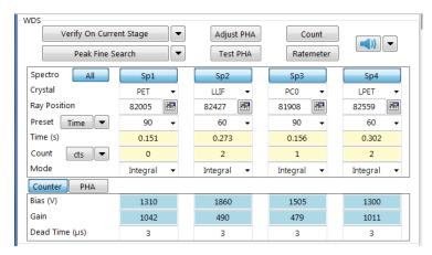
2.0 Using the Position tool on the SX FIVE bar, click on the icon. Make sure the HO6 holder is installed and in the chamber with all of the standards. Refer to sample Exchange SOP.
