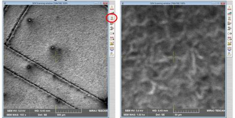
3.6. The specimen now needs to be roughly focused; use the bottom left knob WD on the control panel to focus the image. (<u>note: this adjusts the focus of the objective lens, NOT the actual WD. The stage will not move on the Z direction</u>)
