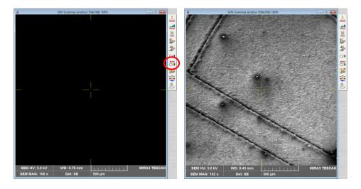
3.5. Next, set the view field to ~200 µm (1 kX Magnification) by turning Mag on the control pad (upper left knob). Look at the magnification values on the bottom of the SEM imaging window.
