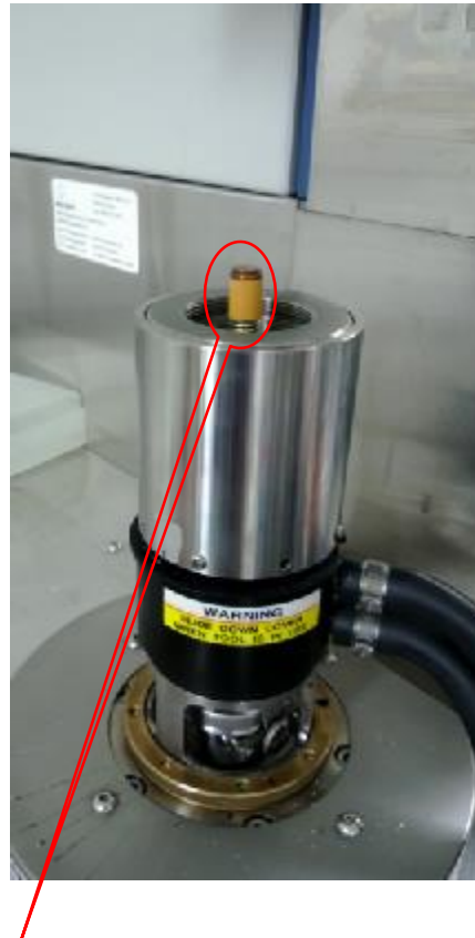
Long PRT Installed
